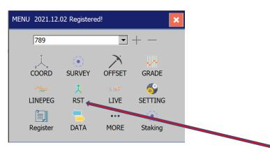
To get the station point from two or more known points select RST from main menu to do a resection. Pick up the reference point from memory or import from SD card. Observe the reference point and press measure button.
