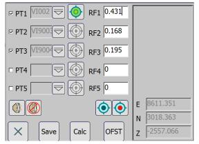
Points that have been measured will have a checked tick box and the measure button will turn green.
