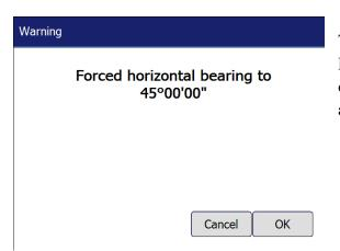
This message confirms that the Horizontal angle will be set to the angle calculated between the occupied point and the backsight point
