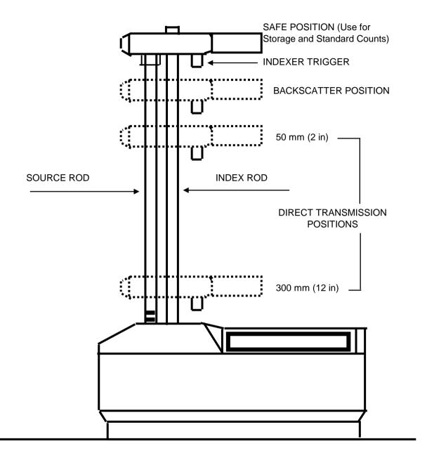
Place the gauge on the reference standard block as shown in Figure 2-2, making sure the block top and gauge base are clean and smooth, with no soil or other material to prevent good surface-to-surface contact. The gauge must be positioned between the raised edges of the block and with the right side of the gauge firmly seated against the metal butt plate on the block.
